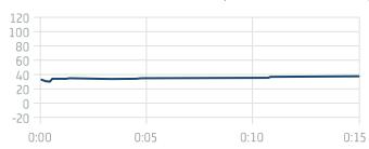
Before you accept or reject the measurement, you can double tap the profile graph to switch between instantaneous and the running average views. If a loud transient noise occurred during the measurement, you can look for the peak in the instantaneous levels and add an exclude marker to that part of the measurement. Otherwise, you can reject the measurement and remeasure.
