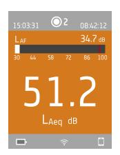
In the middle is the measurement display. There are views for broadband parameters (SLM view and List view), spectrum parameters (Spectrum view), reverberation time measurements (Reverberation time view) and a view for information about your data (About data view).
