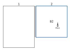
2. Measure the sound pressure level in the receiving room (L2) for the first source position (S1) at each microphone position (R1 to Rn).
