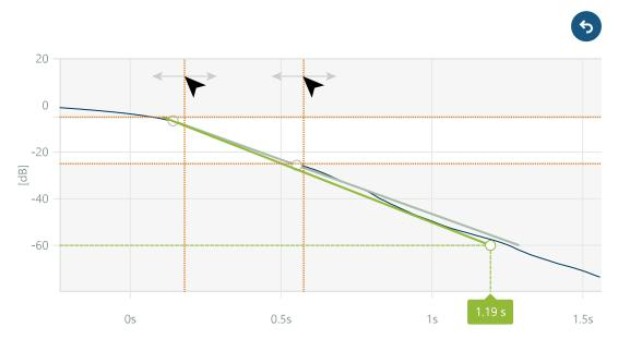
The image above shows which cursors to click and drag to adjust the range. The algorithm-calculated decay curve is still visible (in grey), and you can revert your changes at any time (upper right button).
