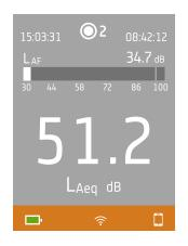
The bottom region provides information about the system: battery, network, and connectivity status.
