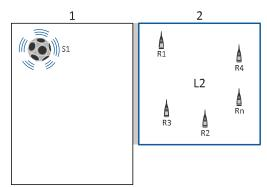
3. Measure the sound pressure level in the source room (L1) for the first source position (S1) at each microphone position (R1 to Rn).
