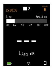
When idle, the instrument displays the current time (to the left) and input settings (to the right).
