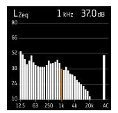
**Spectrum view** displays the frequency analysis of spectrum parameters, shown as decibel (dB) levels by Hertz (Hz).
