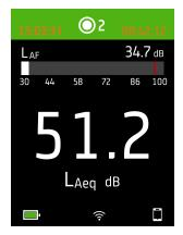
During a measurement, the instrument displays the start time (to the left) and the elapsed time (to the right).
