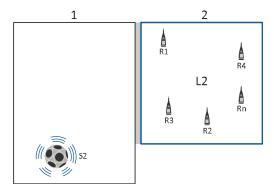
5. Measure the sound pressure level in the source room (L1) for the second source position (S2) at each microphone position (R1 to Rn).
