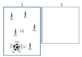
6. Measure the reverberation time in the receiving room (T2) at each microphone position (R1 to Rn).
